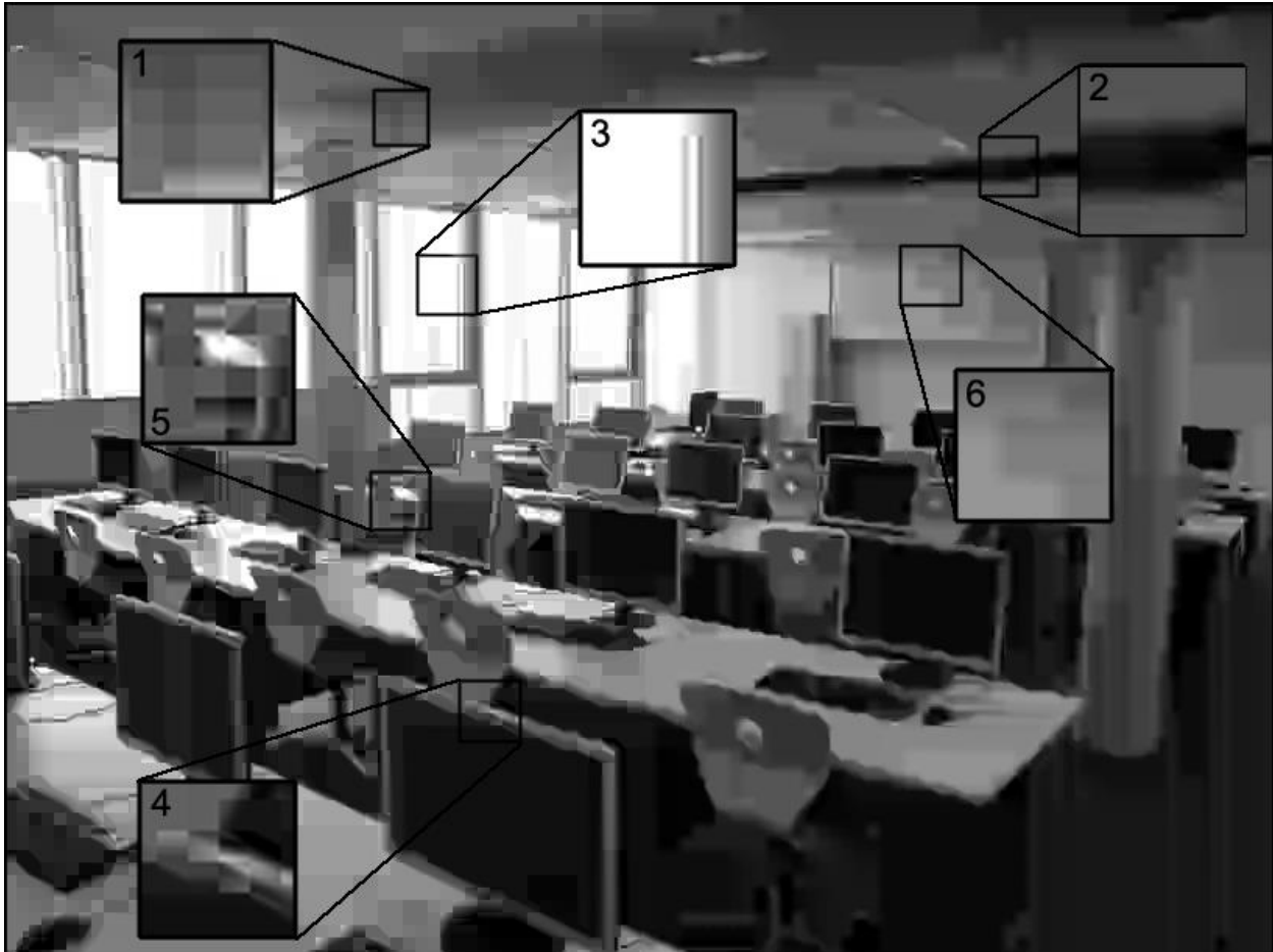
Figure 1: Common artifacts in video coding caused by high quantization and the H.264 deblocking filter (right image part only): blocking at the ceiling (example marked with 1), blurring through deblocking in the right image part (2), ringing at the window borders on the left (3), stair cases at the screens in the front (4), basis patterns between the screens in the middle (5), mosaïking on the white board in the back (6)
