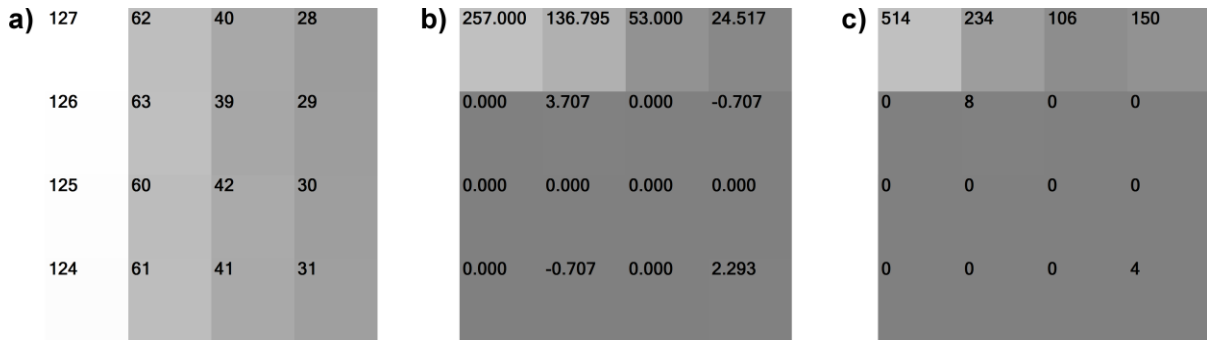
Figure 3: Transform differences between the DCT and the H.264 integer transform: a) Original signal, b) 4x4 DCT transform, c) H.264 4x4 integer transform. Black denotes minimum values, white denotes maximum values; picture domain values are within [-128;127]
