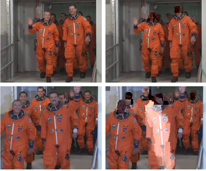
Fig. 8. Left: Frames 46 (top) and 109 (bottom) of the crew sequence with QP 27; right: Encoded with our proposed approach with examples of average drift (28 dB, top) and worst-case drift (14 dB, bottom), respectively, for a high number of scrambled RoIs.
