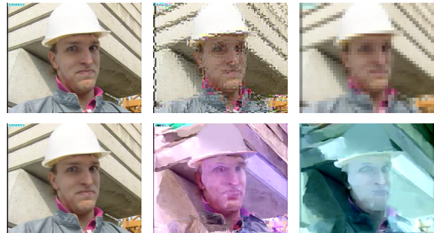
Fig. 1. Examples of compressed (left), encrypted (middle) and attacked images (right): Frame 100 from foreman as JPEG with 75% (top) and H.265/HEVC with randomaccess GOP structure and QP 27 (bottom).
